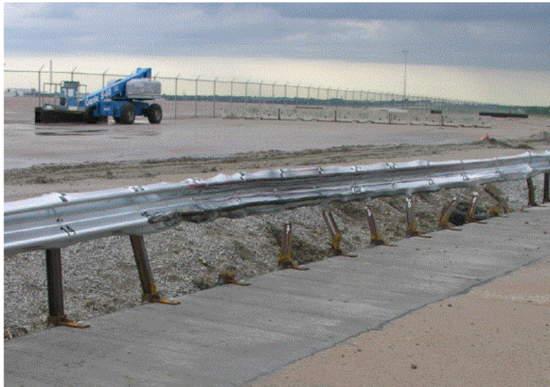
Figure 27: MSG Bridge rail system and vehicle (truck) damages Source: (Thiele, et al. 2011)
