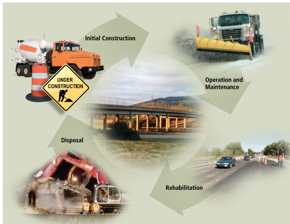
Figure 4: Typical life cycle of bridges
